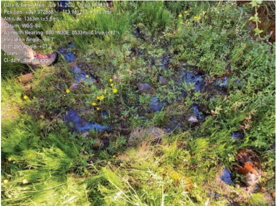
Photograph 1-17 Standing water at the downstream slope toe with petroleum sheen or chelate crystals
